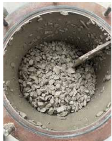
Figure 3 : Aggregate coated with pre-dispersed NGDA
