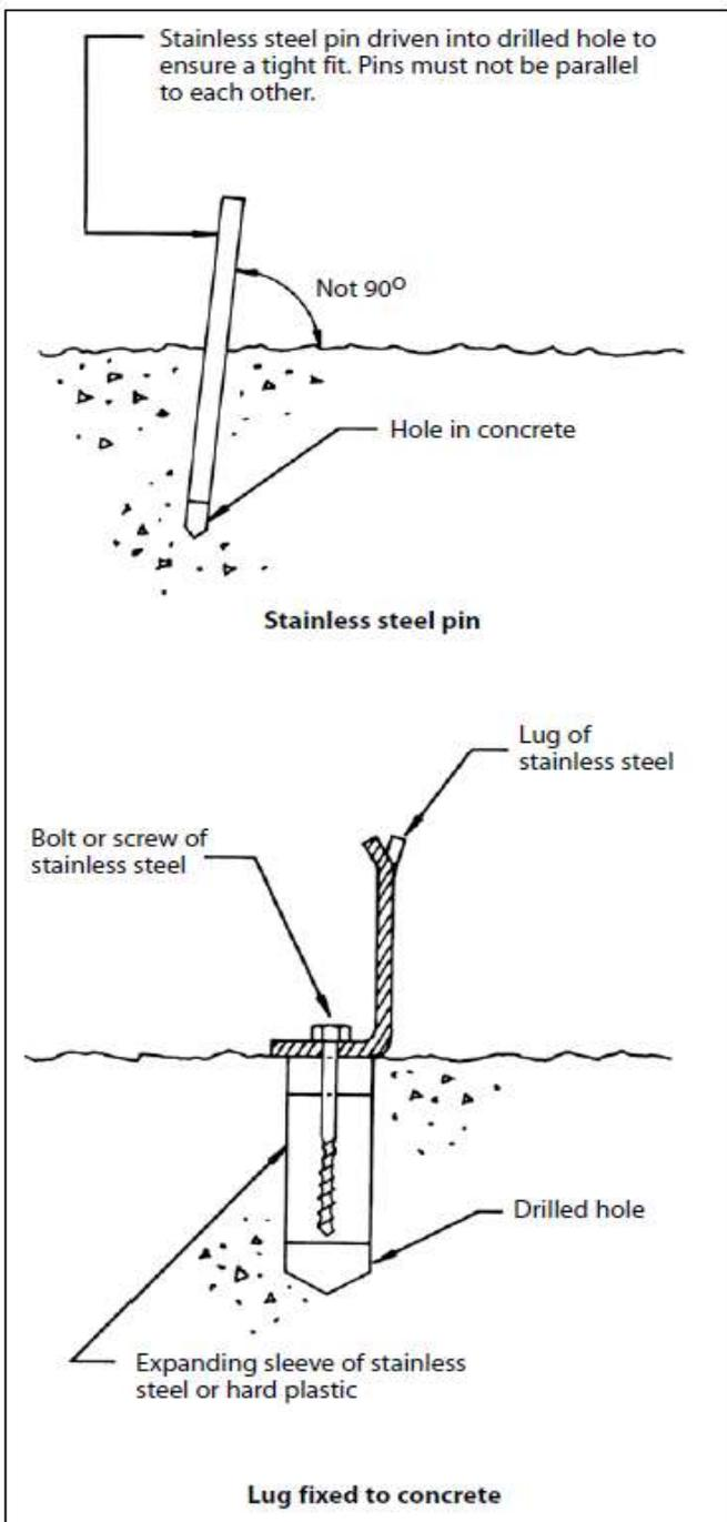
**Figure 2: Mechanical fixing devices**
